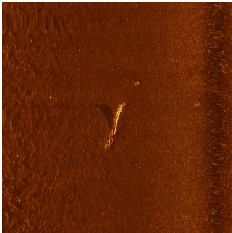
Figure 19. Side-Scan Sonar Target MP 13 / Magnetometer Target MP 11M: Debris and cable
